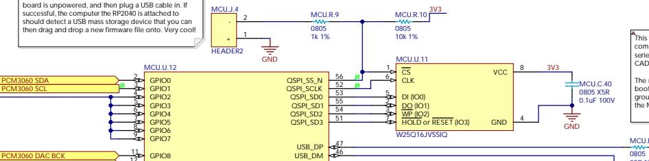
This flash chip holds all of the program memory. The chosen component is a 16MB chip, but smaller ones from the same series could be substituted in to reduce cost (there's about a CAD\$1 difference to be had).
