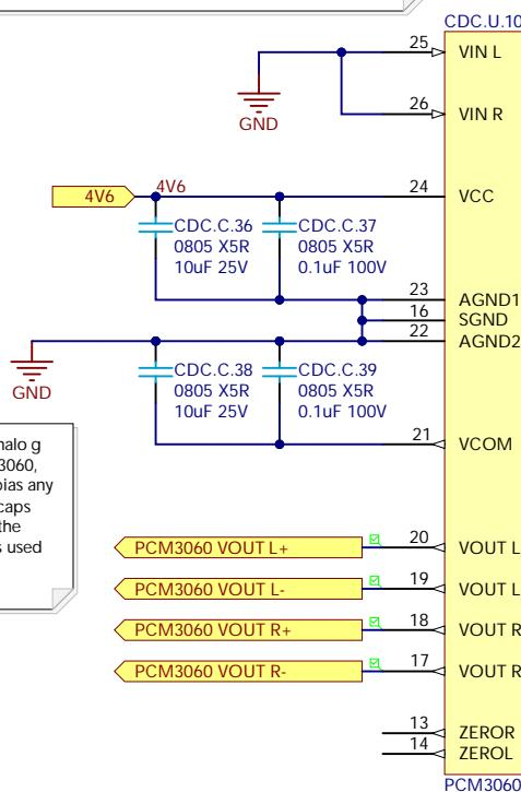
Because we're not using the analog input functionality of the PCM3060, the VCOM pin is not used to bias any external circuitry. The bypass caps mounted here are to stabilize the value of this voltage, since it is used internally to the IC.
