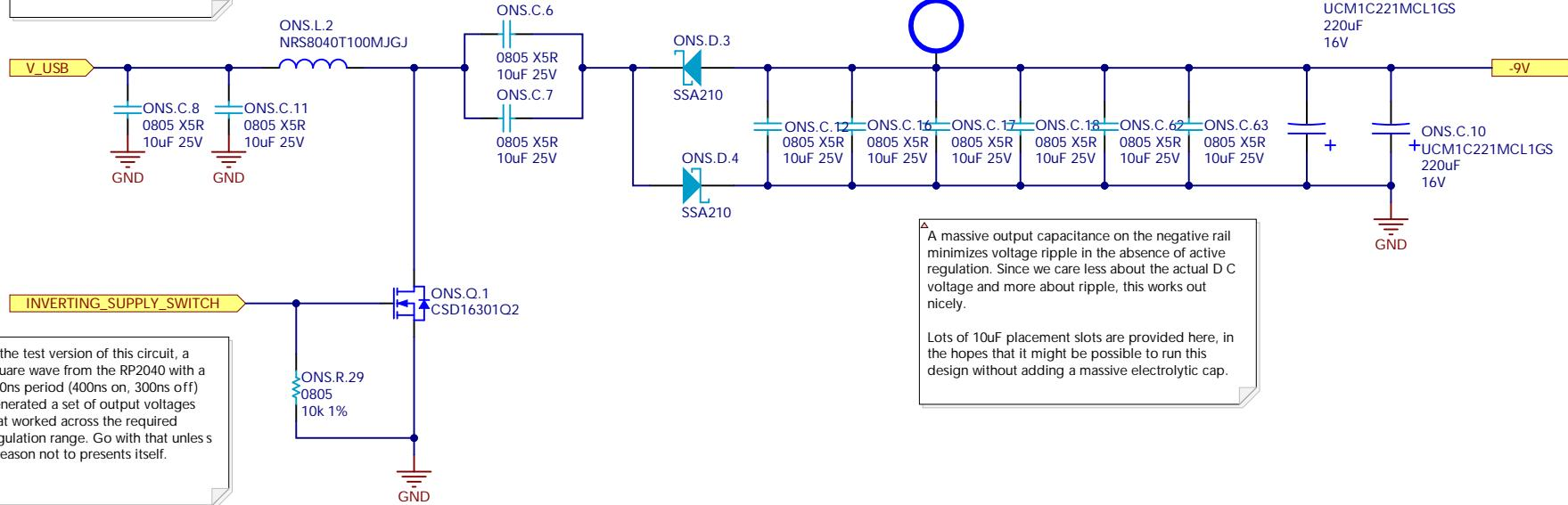
This circuit is pretty freaking weird. It's kind of an unregulated boost converter grafted onto a charge pump.
