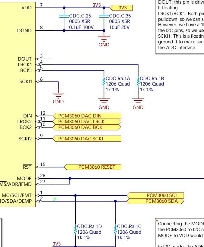
The ADC on the PCM3060 is not used in this application, so it is silly to connect the ADC digital interface pins. However, the disposition of the pins must still be considered. To wit:
