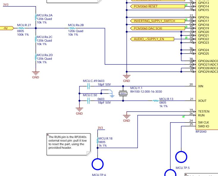
This header provides access to the SWD pins, just in case we need to do some hardcore debugging and/or have to rescue the chip.
