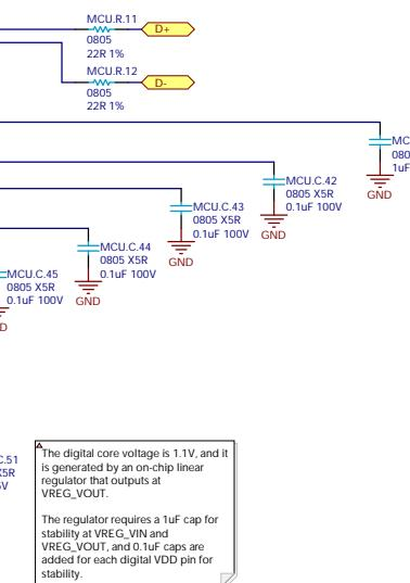
The digital core voltage is 1.1V, and it is generated by an on-chip linear regulator that outputs at VREG\_VOUT.
