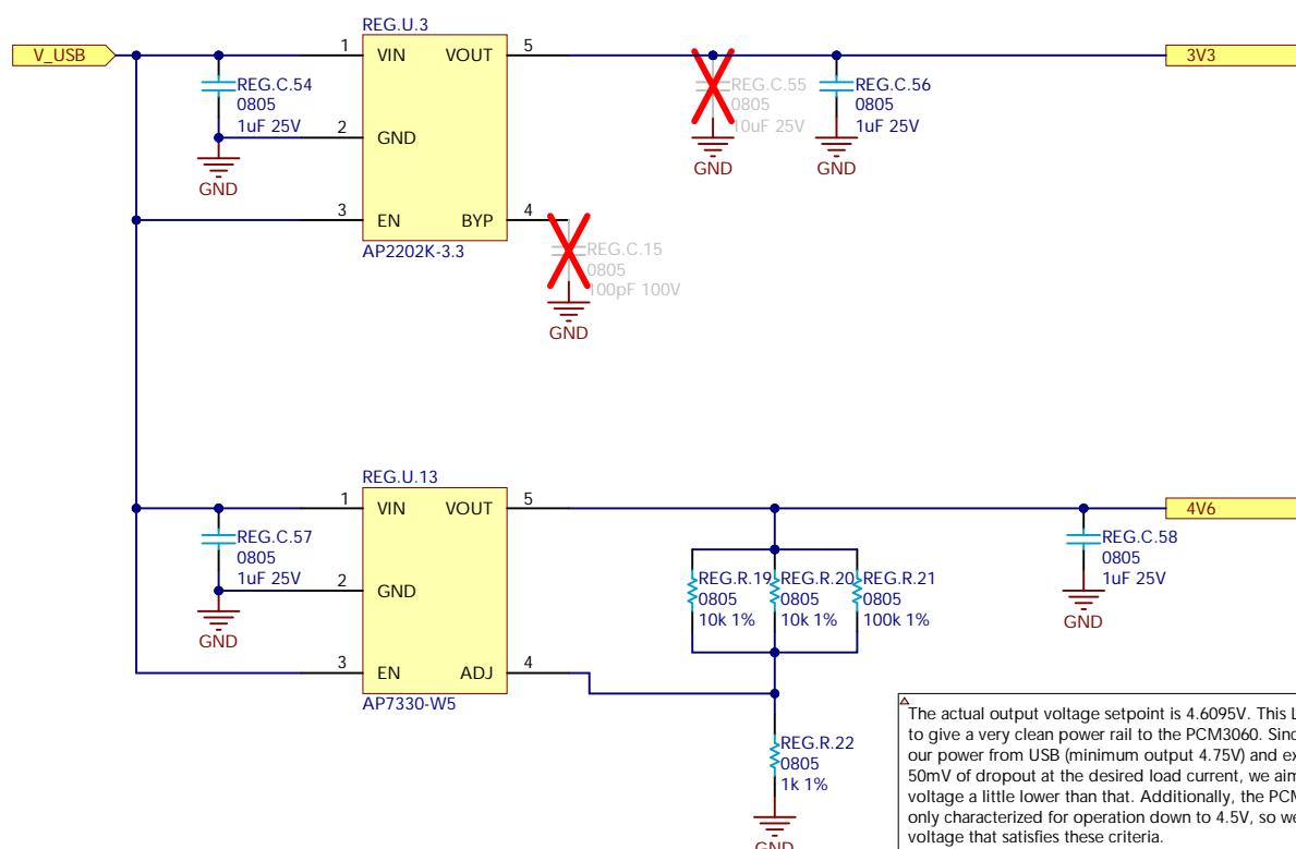
The actual output voltage setpoint is 4.6095V. This LDO exists to give a very clean power rail to the PCM3060. Since we get our power from USB (minimum output 4.75V) and expect 50mV of dropout at the desired load current, we aim for a voltage a little lower than that. Additionally, the PCM3060 is only characterized for operation down to 4.5V, so we pick a voltage that satisfies these criteria.
